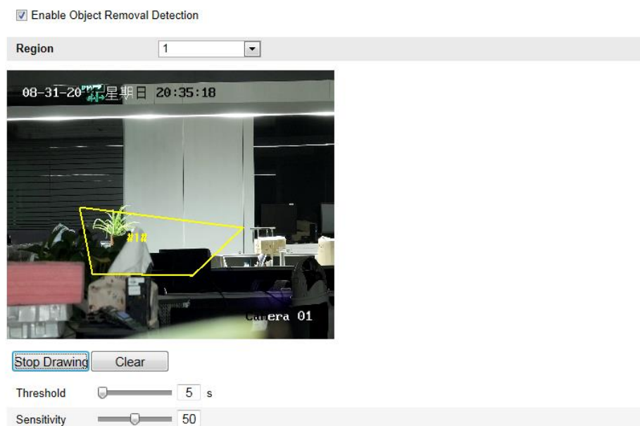
Figure 6-67 Configuring Object Removal Detection
