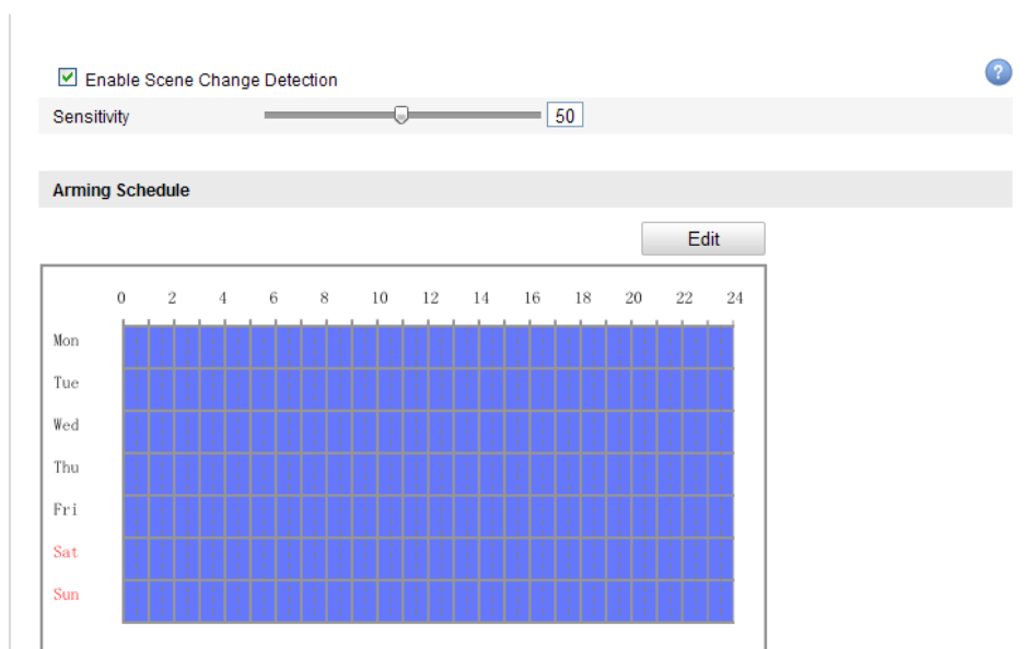
Figure 6-60 Configuring Scene Change Detection
